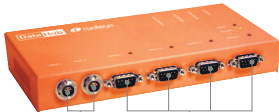
2 x Pt100 Temperature Sensor Ports
